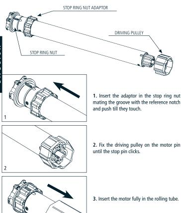
**NB:** If you use tubes with a round form, the driving pulley must be fixed to the tube, and the installation is to be paid by the person who installs the system. For other tube sections the fitting is optional, but strongly recommended.
