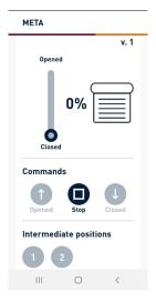
The UP/DOWN/STOP buttons in the control panel allow to Open/Close/Stop the rolling shutter.
