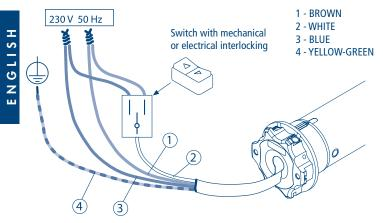
From white wire it's possible to control the motor in the middle position:
