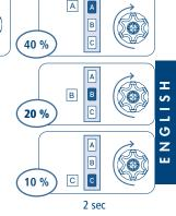
The OPEN ZRX is factory set to a closing force of 20 % of the nominal torque. This force can be changed very easily by the remote control. It can be reduced by 10 % or increased up to 40 %, depending on the desired result.
