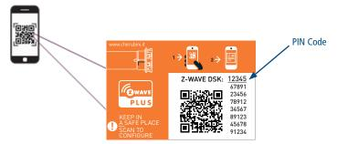
The PIN code of the Z-Wave Device Specific Key (DSK) is required when adding the OPEN ZRX to a Z-Wave network with a controller supporting Security 2 Autenticated (S2). The unique DSK code is printed on the product label. The first five digits of the key are highlighted and underlined to help the user identify the PIN code portion of the DSK text.
