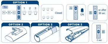
Remove one battery and wait minimum 5 seconds or press any button.
