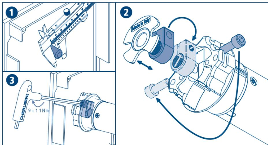
**1** The bolt has to be in aluminum with minimal  $\varnothing$  11,5 and maximal  $\varnothing$  11,9 mm.
