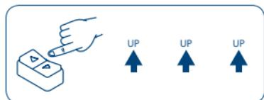
**Attention!** If the sequence requires a repetition of the same commands (Up+Up/ Down+Down), an interposition of the Stop position could be necessary depending on the type of switch in use.
